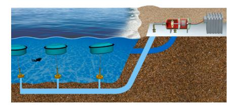
pump that moves pressurised water along pipes to the land. This water powers a turbine (the same as in a hydropower plant) which runs a generator that produces electricity. See page 2 for a diagram showing this process.
